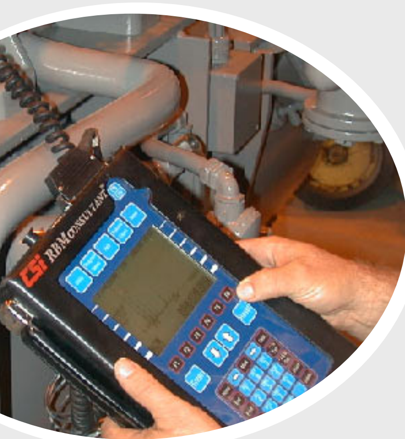
A hand-held data collection unit is used to analyze readings at various vibration survey points on the motor and compressor.
